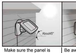
Make sure the panel is 45°from the horizontal level. This angle can be adjusted.
